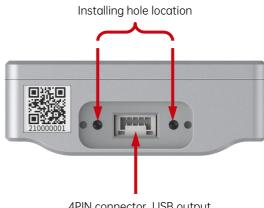
4PIN connector, USB output
